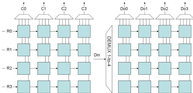
Fig. 4. Transpose RAM (left) and DC RAM (right).
