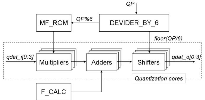
Fig. 5. Quantizer architecture.
