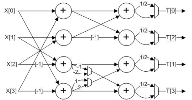
Fig. 2. Hybrid 1-D transform architecture for integer DCT-based and Hadamard transforms
