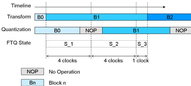
Fig. 8. Three states of pipeline operation.
