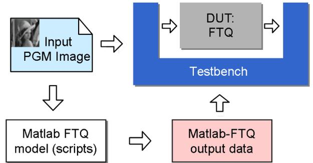
Fig. 9. Verification model for the design.
