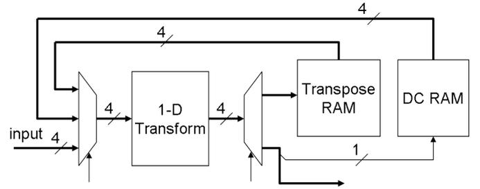
Fig. 3. Architecture of forward transform.
