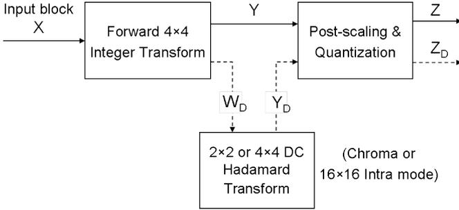
Fig. 1. Transform and quantization flow diagram.
