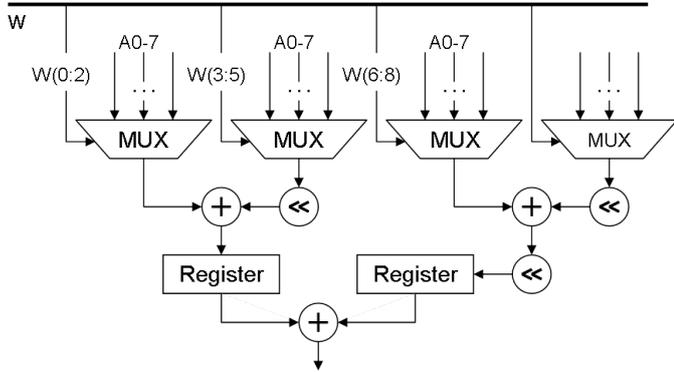
Fig. 7. Multiplier for quantizer using the pre-multiplier element.
