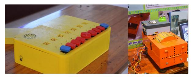
Figure 5: Text reading device for the blind
