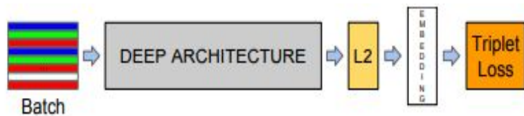
Figure 2. Model structure. Our network consists of a batch input layer and a deep CNN followed by L_2 normalization, which results in the face embedding. This is followed by the triplet loss during training.
