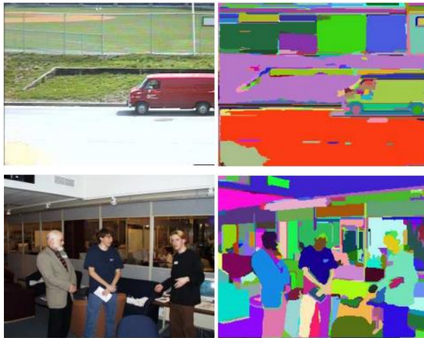
Outdoor & indoor scene segmentation results produced by Felzenszwalb's algorithm
