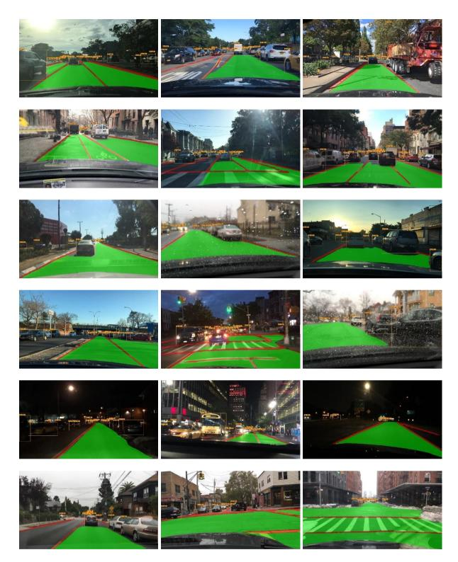
Figure 10: Multi-task results using HybridNets. The red lines are the lane lines, the green areas are the drivable area, and the orange bounding boxes are traffic objects.
