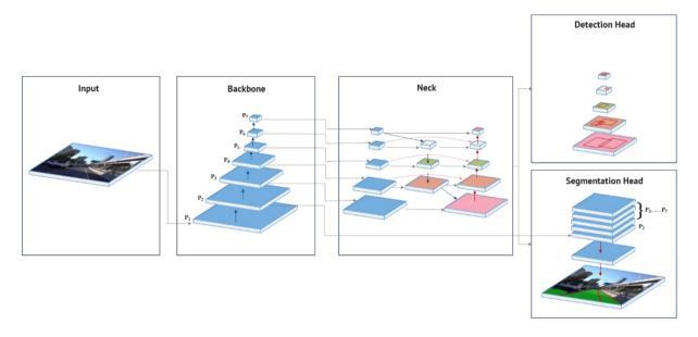
Figure 2: HybridNets Architecture. It consists of one encoder: backbone network and neck network; and two decoders: Detection Head and Segmentation Head. The backbone network generated 5 feature maps from  $P_1$  to  $P_5$ . By down-sampling the feature map  $P_5$ , we obtain two feature maps  $P_6$  and  $P_7$ .
