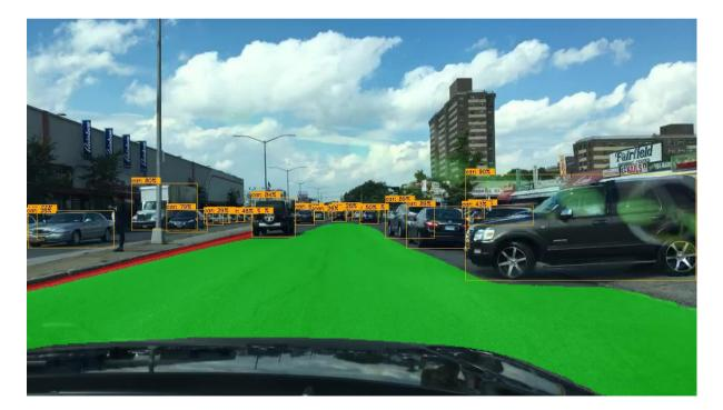
Figure 1: Results for inference of HybridNets. Our proposed network performs three tasks, including traffic object detection, drivable area segmentation and lane line detection. The green areas indicate the drivable area, the blue lines are the lane lines, and the orange boxes are the traffic objects.
