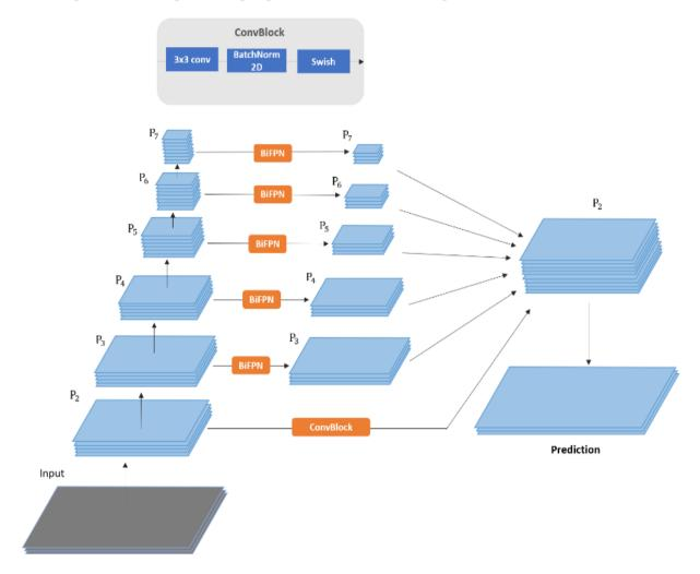
Figure 3: The Segmentation branch of HybridNets architecture.
