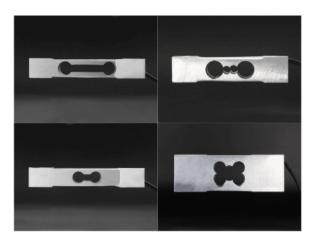
Figure 13: Bar-type load cell
