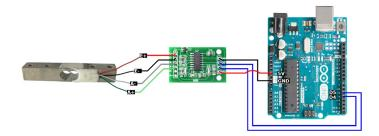
The weight value is generated in a separate setting using the Arduino IDE and a third-party application called CoolTerm. Weight value transmitting from the Arduino Uno and the scale to the serial port captured by CoolTerm. The output is obtained in a .txt file for further processing.
