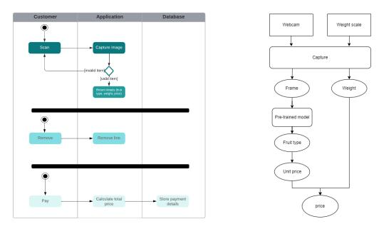
Figure 14: Application workflow and Price calculating progress
