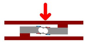
The weight scale base is 3D-printed, and the following design is capable of measuring objects equal to or below 10kg.
