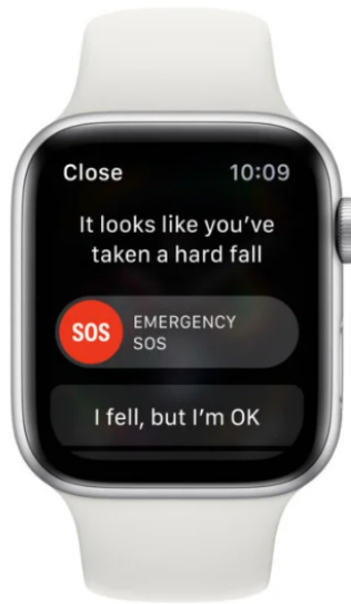
Figure 1. An example of fall detection on the Apple Watch [2].
