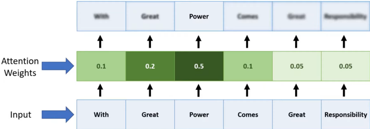
Figure 5. An example of assigning different weights to each input in a data sequence [10].
