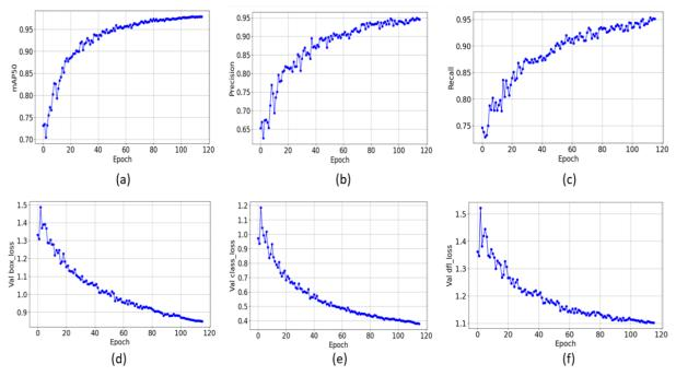
Figure 15. Training result (a). mAP (b). Precision (c). Recall (d). Val box\_loss (e). Val class\_loss (f). Val dfl\_loss
