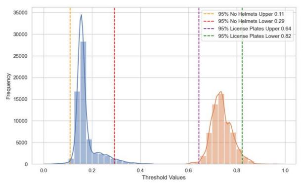
Figure 8. Histogram of threshold values for no\_helmet and license plate
