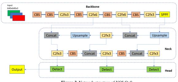
Figure 3. Network structure of YOLOv8
