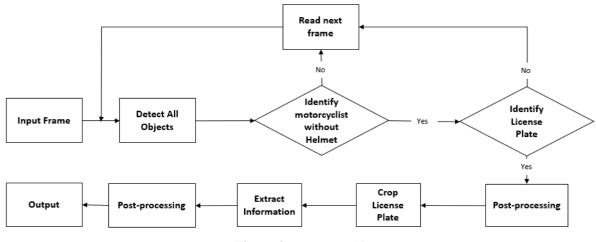
Figure 2. System architecture
